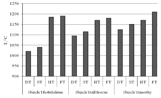
Fig. 4. Comparison of the ash melting temperature of birch and tall fescue, festulolium and timothy biomass pellets (1/3)
