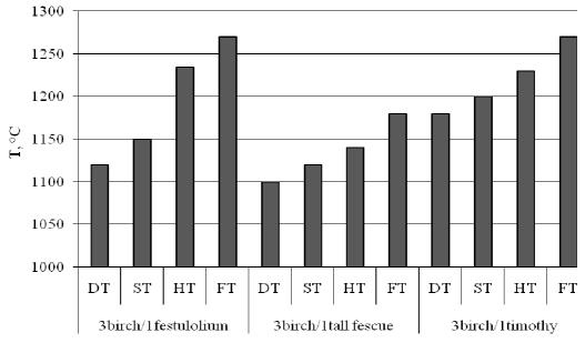
Fig. 2. Comparison of the ash melting temperature of birch and tall fescue, festulolium and timothy biomass pellets (3/1)
