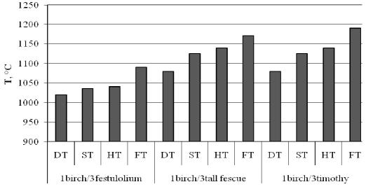
Fig. 3. Comparison of the ash melting temperature of birch and tall fescue, festulolium and timothy biomass pellets (1/1)
